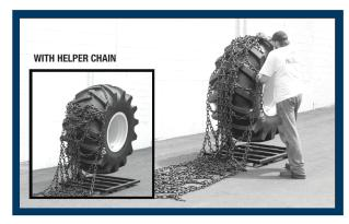
Pull a portion of the chain over the tire and use the tire lugs to help hold the chain in place. A helper chain or rope may also be used (see inset). Move the machine forward to bring the chain over the tire, spreading the Diamond or Ring sections apart to cover the width of the tire. Rotate until the chains can be connected at the centers.
