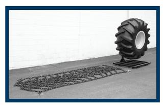
Lay chains out flat behind tire with studs (Diamond® chains) or lugs (Ring chains) facing upwards. Spread the chain apart lengthwise and position it so that it will be centered on the tire.
