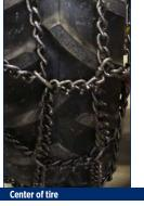
4B. Pull tail chains tight through connecting ring.
