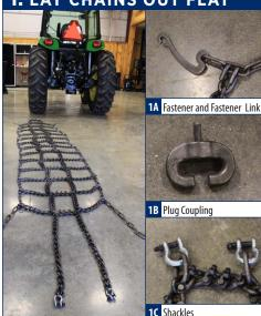
Lay chains out flat behind tractor making sure ends of cross chain hooks are facing up. Remove all twist and tangles.
