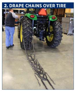
Drape chains over tire in the same position making sure ends of cross chain hooks face up and away from tire. Center chains on tire and position them to touch the ground in front of the tire. Tuck first cross chain under tire a bit in preparation to roll over them.
