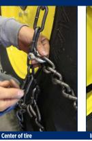
4C. Pull tail chain to tighten. Connect shackle on tail chain to side chain.
