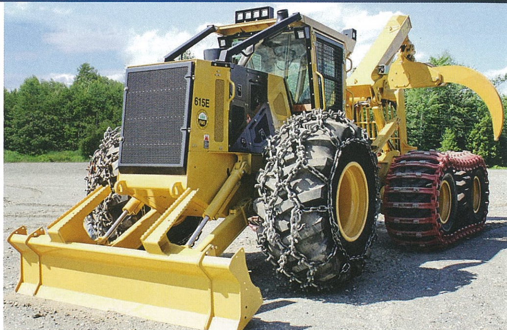
Tigercat 615E six-wheel skidder outfitted with heavy duty BABAC 7/8 in 1.5 Diamond Chains and Clark Tracks
