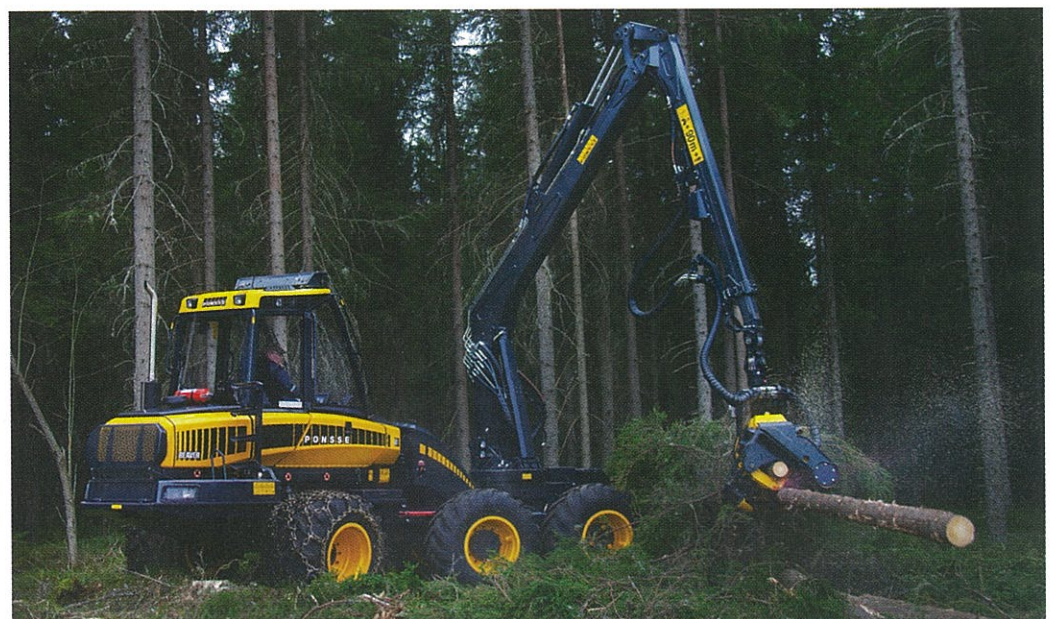
Ponsse Beaver harvesting on BABAC Triple Diamond Euro chains for tyre protection and constant traction
