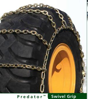
**Predator Swivel Grip** ladder style chains have the same great features and construction as the Predator Skid Steer, plus a Swivel hook (*below*) to allow for easy installation of cross chains while the chain is still on the tire.
