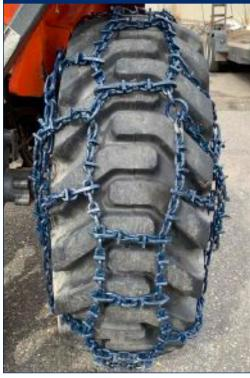
Test Drive, Inspect, Re-Tighten tire chains by **REPEATING STEPS 4A- 4D** so chains fit snug around the tire. Make sure the quick hook and fastener are secure.
