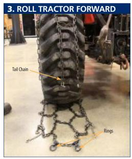
Roll equipment forward until the end of the chains are at a good working height—approximately axle height.
