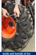
**4B.** Connect fastener on inside the tire. Count the same number of links on the outer side chain and place end of fastener through that link.
