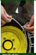
4B. Count the same number of links on the outer side chain and place end of fastener through that link.
