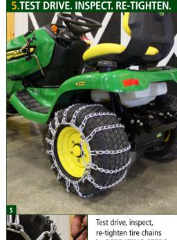
by REPEATING STEPS 4A- 4D so chains fit snug around the tire. Make sure the quick hook and fastener are secure. Attach extra links back to the side chain with heavy duty cable ties (5A).
