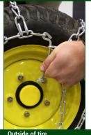
4C. Fold fastener back toward side chain to tighten. To increase tension, place fastener one link lower and fold back. Retighten inner guick hook.
