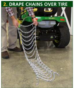
Drape chains over tire in the same position making sure ends of cross chain hooks face up and away from tire. Position chains to touch the ground in front of the tire and tuck first cross chain under tire a bit in preparation to roll over them.
