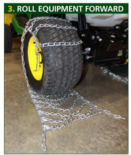
Roll equipment over chains until the quick hook and fastener are positioned midway on the tire and both side chain ends are easily accessible. Adjust chains to be centered on tire treads.
