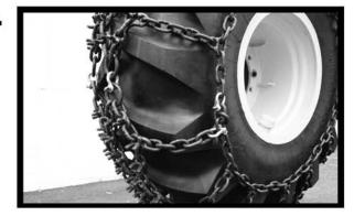
Connect the free cross chains to evenly spaced links on the side chain and then connect the side chains together. Be sure to tighten equally to ensure proper fit.
