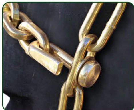
Swivel hooks on the end of the cross chains allow for easy installation of replacement cross chains.
